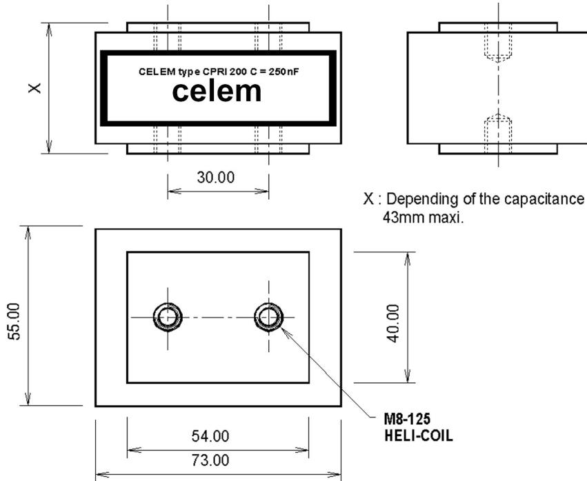
The CPRI 200 mica conduction-cooled capacitor provides 250kVAr at ultra-high frequencies (up to 100MHz) and high ambient temperatures (up to 150C). The CPRI 200 can be manufactured to order with the capacitance of the customer's choice. The values in the attached table are typical of the range of available values.
