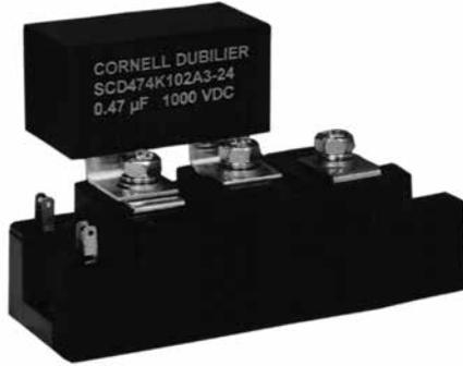
Style SCD offers protection against voltage transients in low to medium current IGBT applications where high dV/dt is encountered. Connect these capacitors from C1 to E2 on a dual IGBT module or from P to N on a six-pack module to eliminate severe voltage transients. Parts ending with Z25 fit IGBTs with 23mm, 25mm and 28mm lead spacing. If you have a preferred lead spacing, please specify.
